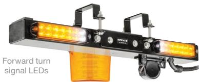
Forward turn signal LEDs
